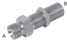
BSPP Male x BSPP Male Extended Bulkhead 60° Cone c/w Locknut
