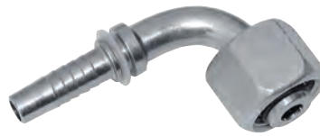
90° Metric Female 24° Cone Seat, S Series, DIN 3865
