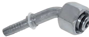
45° Metric Female 24° Cone Seat, S Series, DIN 3865
