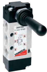
G1/8", 5/3 CC Lever Valve Bistable
